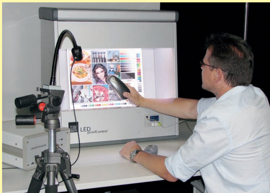
Measuring the lighting conditions at the customer with a spectrophotometer and simulating this environment within the new LED Proofcontrol cabin, as demonstrated by Just Managing Director Michael Gall. This is an invaluable capability.
